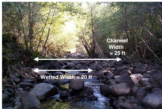
Figure 9.10 The Channel width and wetted width.
