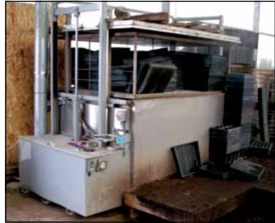
Fig. 7.2.2. — Apparatus for submerging flats, trays and small containers in hot water.
