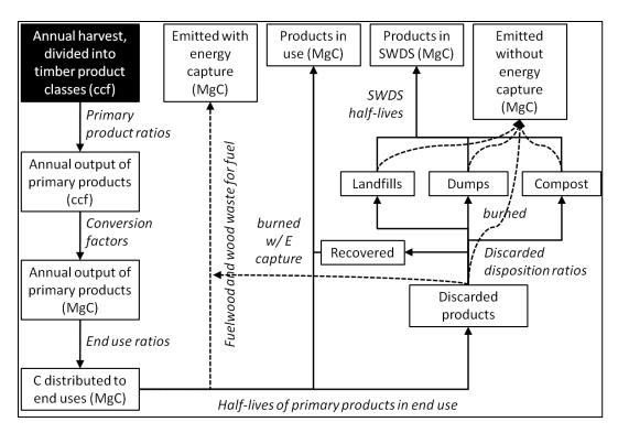
Figure 1. Diagram of the harvested wood products (HWP) model used to quantify Oregon carbon storage and emissions (from Stockmann et al. 2012).
