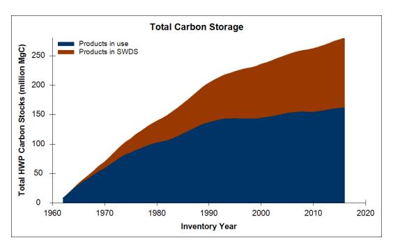
Figure 3. Cumulative HWP C stock as products in use and at solid waste disposal sites (SWDS) from timber harvested in Oregon 1962-2017.
