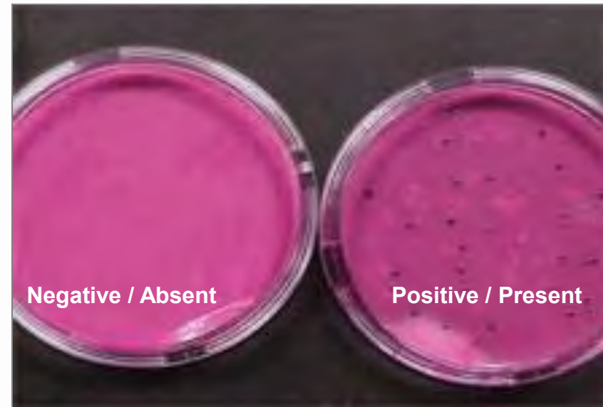
Negative coliform test on the left and positive on the right
