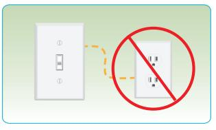
Do not use outlets that are controlled by wall switches.
