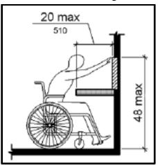
**Unobstructed** side reach shall be between 15" to 48" in height from the floor.
