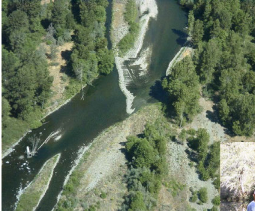
Bridgepoint Push-Up Dam (2001) Push-Up Dam on the Applegate River Used for Agricultural Purposes
