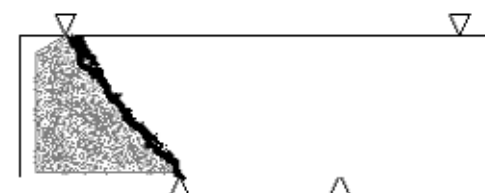
Figure B.6.3.3: Typical failure modes for CMI/Reichhold beams reinforced for flexure and shear at 45 degrees.
