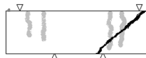
Figure B.2.2.3: Typical failure modes for MBrace™ carbon flexure and shear at 90° reinforced beams.
