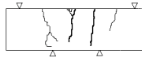
Figure B.6.2.3: Typical failure modes for CMI/Reichhold beams reinforced for flexure and shear at 90 degrees.
