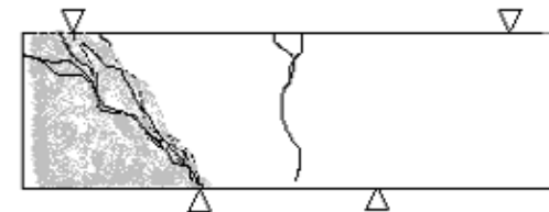
Figure B.8.2.3: Typical cracking and failure modes for beams reinforced with the Tyfo® glass system for flexure and shear.
