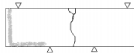
Figure B.5.2.3: Typical crack patterns and failure modes for beams reinforced with Tyfo® carbon for flexure and shear.
