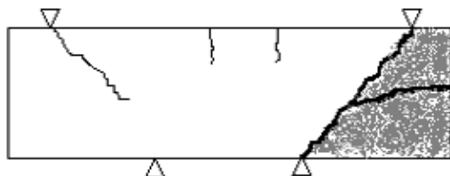
Figure B.6.1.3: Typical failure modes for CMI/Reichhold beams reinforced for flexure.
